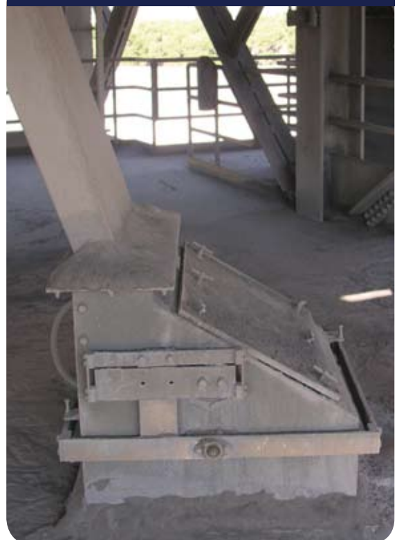
DLM Solids Flow Meter with a curved measuring chute receives material free of impact
