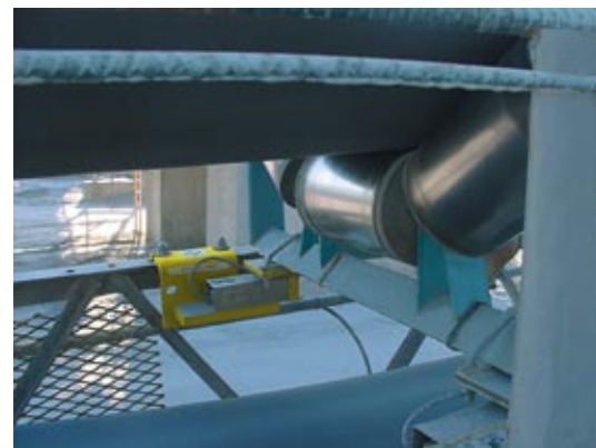
BEMP™ Belt Scale in an aggregate industry installation.
