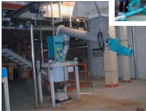
Figure 4a: Coriolis feeding system with feed screws for additives
