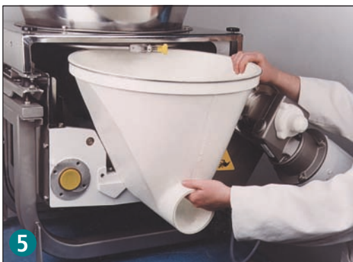
5 Hopper slides out for easy cleaning, replacement or maintenance.
