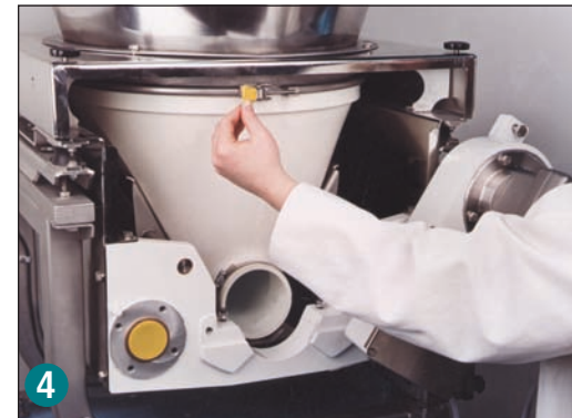
4 Release band clamp lever for hopper removal.
