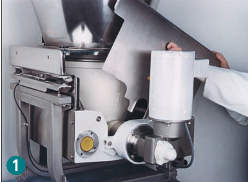
1 All components are accessible from the rear of the feeder instead of the discharge side. Simply remove back panel and loosen bolt.
