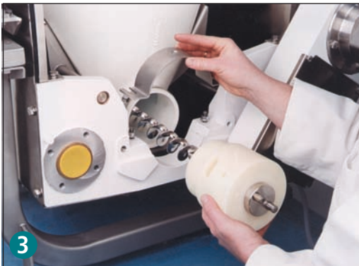
3 Helix is easily removed allowing for quick helix style and diameter changes.
