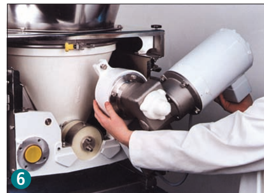
6 Reposition motor and drive assembly. Tighten bolt and you're ready to run – all in under two minutes.
