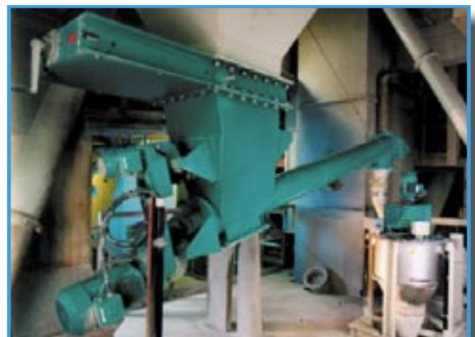
Figure 8b and 8b: Coriolis feeding systems with inclined feed screws for gypsum and stucco.
