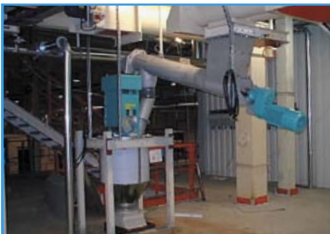
Figure 8b and 8b: Coriolis feeding systems with inclined feed screws for gypsum and stucco.
