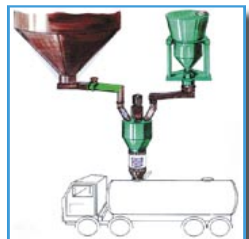
Figure 6: Coriolis loading station.
