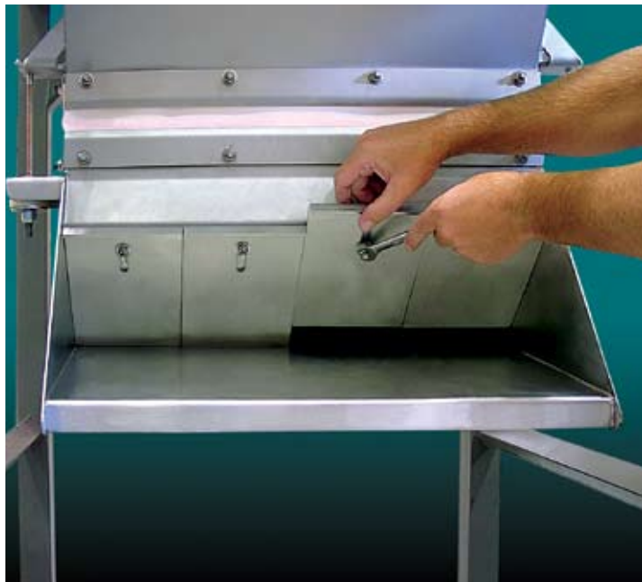
Gap adjustment can be easily made by simply using a wrench.
